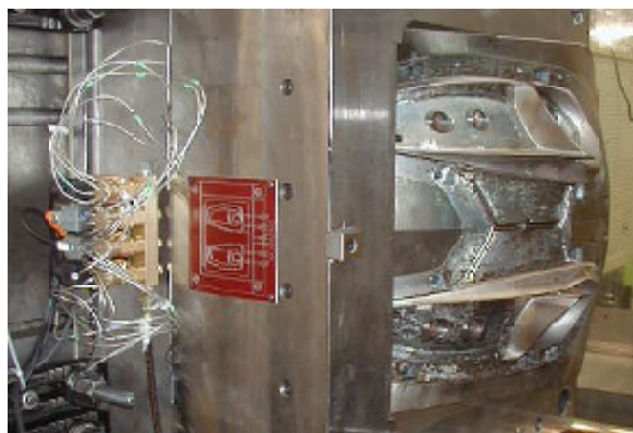
Mold with CO 2 -temperaturare control
