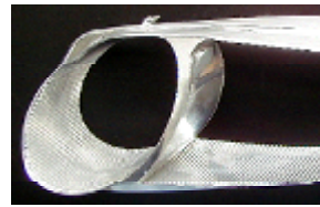
Part with thin fillet and CO 2 -temperature control
